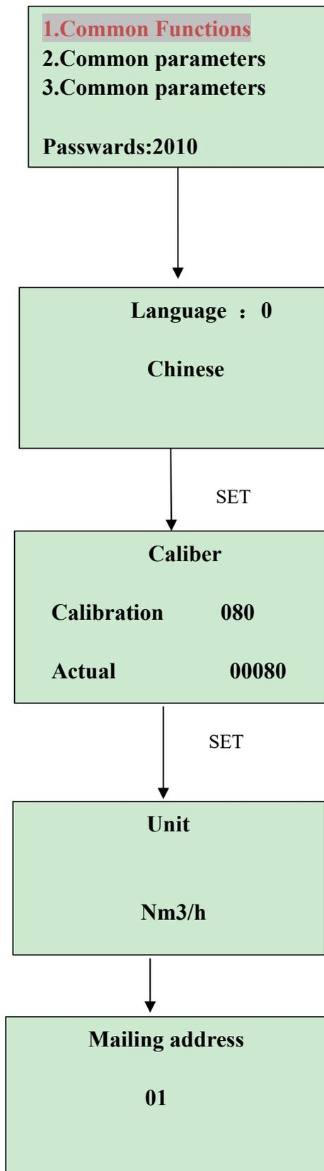
In the main interface, press the SHFIT key to enter the main menu interface. Press the SET key to move the cursor to the password, then press the ▲ key to change the corresponding password, and then press the SET key again to shift, and enter the password 2010 in sequence.
