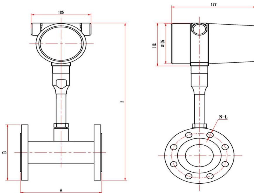
Figure 4 Flanged flow meter
